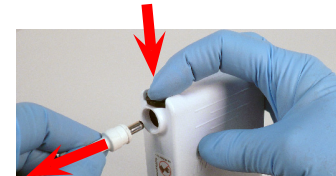
8. Disconnect Power Cord from the Battery - push Secure Connection Button down, pull Cord Connector out, release the Button.
