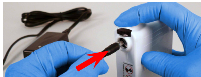
10. Connect Charger to safe power source; connect Charger Cord Connector into Battery Receptacle until fully seated.
