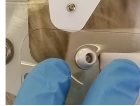
9. Attach (snap) one side Hood-Lens mounting hole to respective Helmet side mounting post. Repeat on other side.
