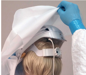
7. Holding the Helmet securely on head, grasp back bottom of Hood Skirt and pull up, over, and down below Helmet in back.
