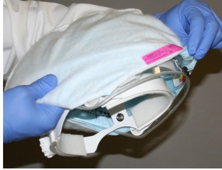
2. Pull the front of the Filter down over the front of the Helmet, pulling the Filter alignment hole over the center Helmet alignment post of the Helmet.
