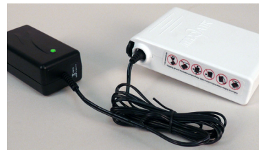
11. Connect the Battery to a powered on Charger.
