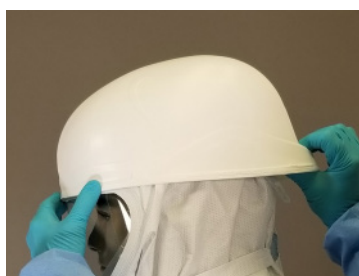
3. While holding the HFR FCC in place in front, continue pulling the it down in back until its back bottom is just below the back bottom of the Helmet.
