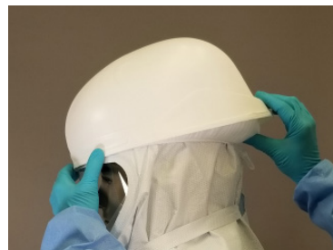
2. Using the thumb under the back bottom of the Helmet, pull the top back of the HFR FCC down onto the Helmet and HLF.
