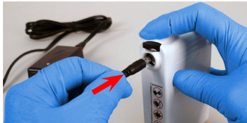
5. With the Charger connected to the mains wall power, connect the Charger Cord to the Battery. Push the Charger Cord Connector into the Battery Receptacle until it is fully seated.
