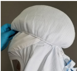
1. Initiate donning the HLF (Heavy Loading Filter) by tucking its back bottom up under back bottom of Helmet.
