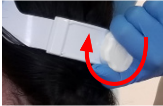
14. Tighten Ratchet Knob (clockwise) as tight as possible without causing discomfort to secure Helmet on head for all anticipated activities.
