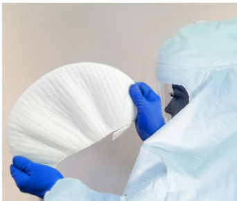
1. Initiate donning the HLF (Heavy Loading Filter) by tucking its back bottom up under back bottom of Helmet
