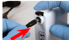
3. Connect Charger to a safe power source, then connect Charger to Battery by pushing its Cord Connector into Battery Receptacle until fully seated.
